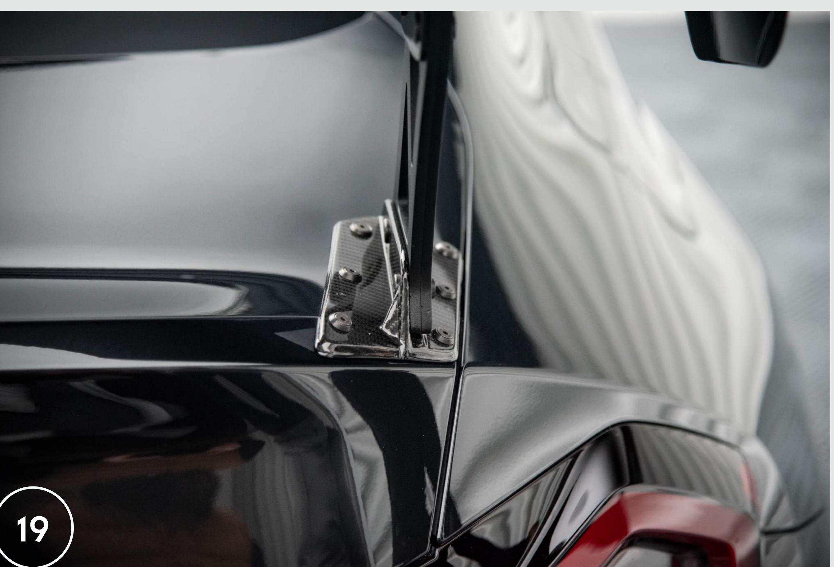
20. Screw both parts together, apply low-tear safety adhesive to the screw threads.
